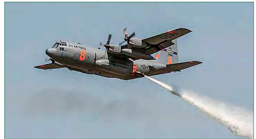
North Carolina Air National Guard C-130H from the 153rd Airlift Wing, utilizing Modular Airborne Firefighting System (MAFFS), 2 May 2015. (Photo: US Air Force, MSgt Charles Delano)
